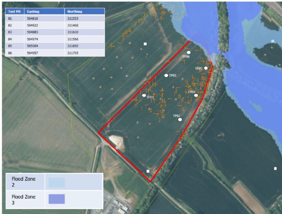
Plate 1: Surface Water Flow Routes and Test Pits (redline – substation outline, green line – flow route model boundary)
